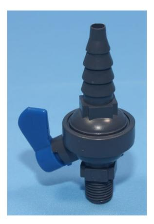
To be utilized with the GAS GA-MA Beaker. Each PVC valve has four o-rings, 1/4" NPT threaded end and a tapered hose connection for a flexible tubing
